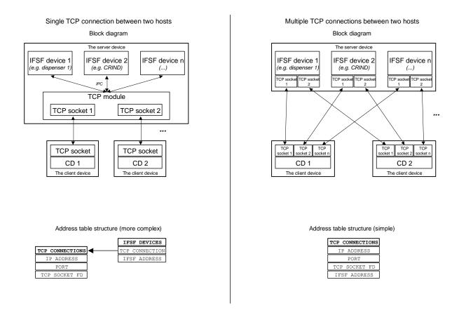
Figure 3: The two possible architectures of the TCP connections created among IFSF devices
