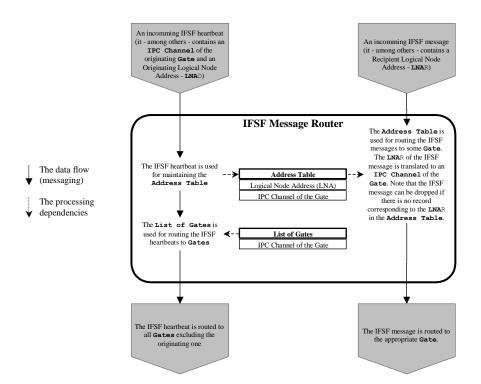
Figure 2: The structure of the IFSF Message Router module 12.3.2 IFSF TCP/IP Gate module
