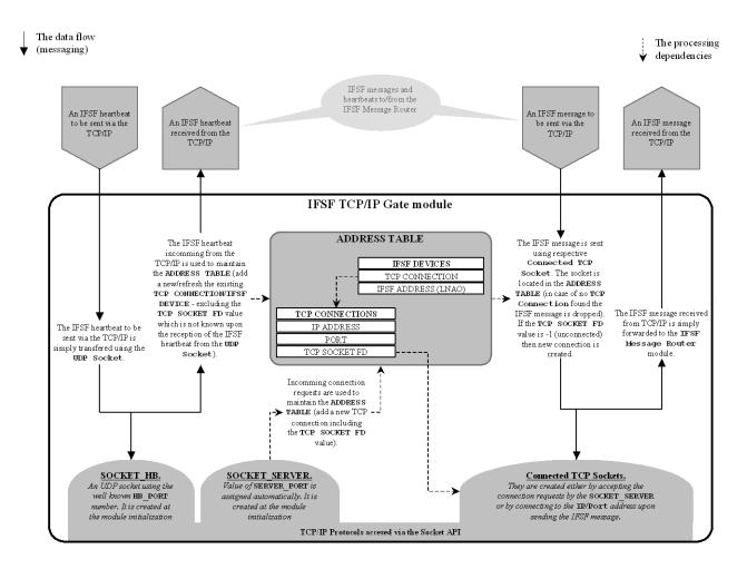
Figure 5: The detailed structure of the IFSF TCP/IP Gate module
